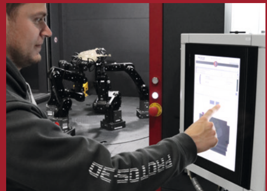
PRAFS-HMI control panel: direct access to all stored PRAFS setups (several thousand possible)
